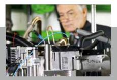
As well as the new technology used for the burning process, in the new Hydronic 2 Commercial and Hydronic M 2 water heaters the fan has also been further developed, and is now driven for the first time by a brushless motor. This electronically commutated motor (ECM) technology guarantees maximum running times.
